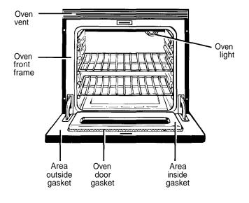
3. Clean spatters or soil on the oven front frame and the oven door outside the gasket with a dampened cloth. The oven front frame and the oven door outside the gasket do not get cleaned by the selfclean cycle. On these areas, use detergent and hot water or a soap-filled steel wool pad. Rinse well with a vinegar and water solution. This will help prevent a brown residue from forming when the oven is heated. Buff these areas with a dry cloth. Do not clean the gasket.
